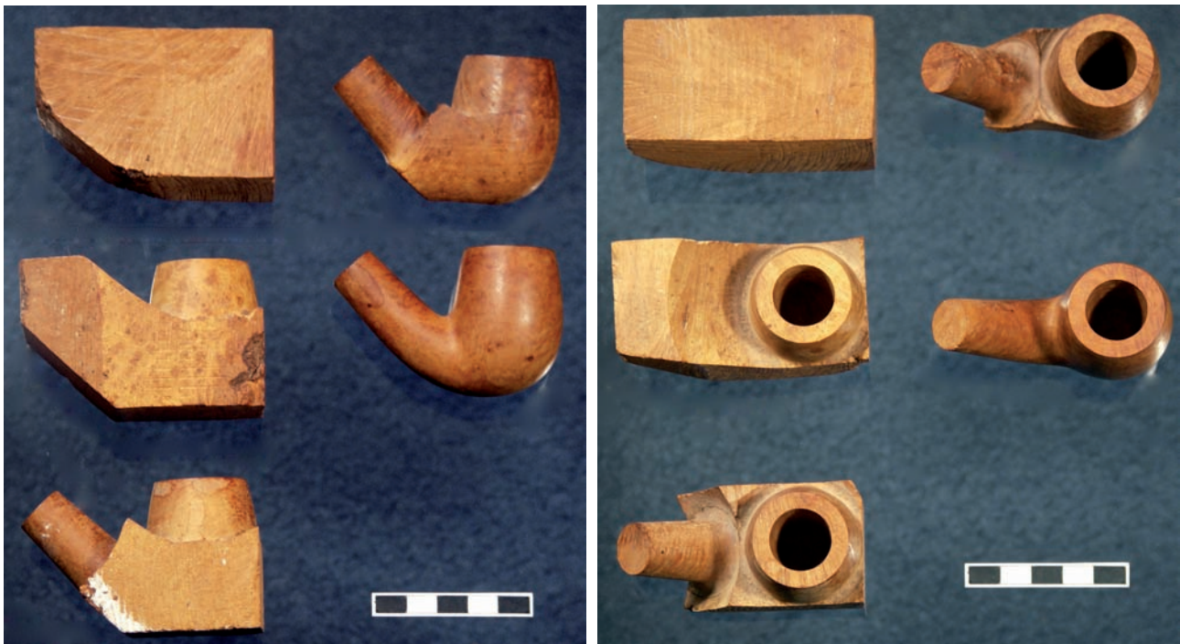
Figure 8: Five stages in the production of a bent billiard pipe, as viewed from the side (left) and above (right). The actual objects are in the National Pipe Archive (LIVNP:2010.19; photographs by S. D. White).
