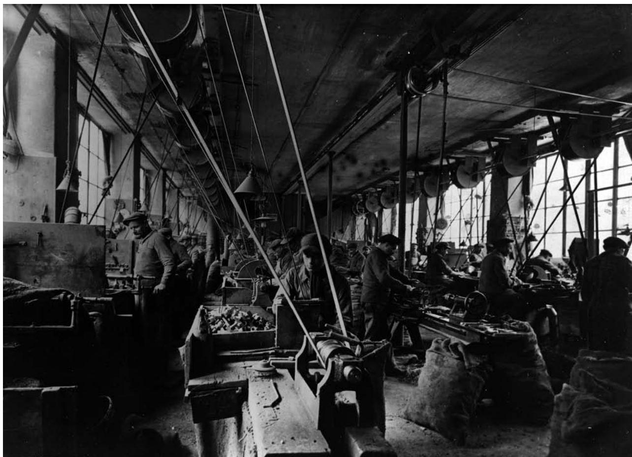
Figure 7: Belt driven lathes turning bowls at the La Bruyère factory c1920 (photograph courtesy of the John Adler Archive).
